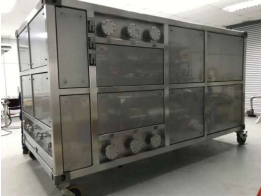
Figure 6. Heat exchanger block (with HX 2/3/4).
