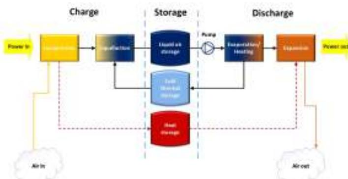
Fig. 2. Process flow diagram of liquid air energy storage plant (Giacomini et al. 2011).
